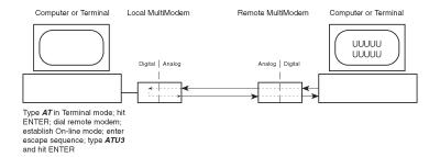
Figure 6-2. Digital Loopback Test (local/manual)
